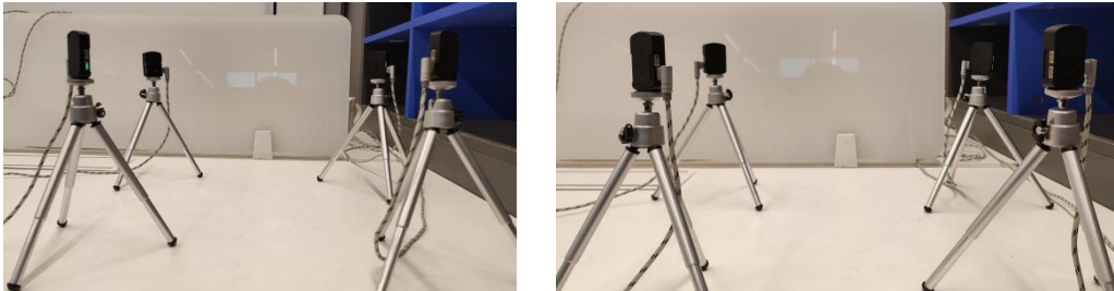
Fig. 1: The physical picture of the installation direction of the LTS anchor antenna. Left: antenna facing inward; right: antenna facing outward
